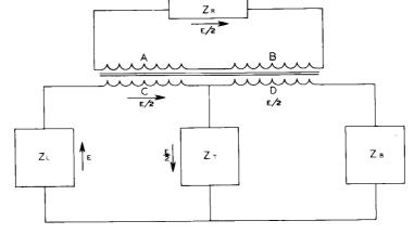
$Z_1$  = Telephone line impedance  $Z_k$  = Balance network
