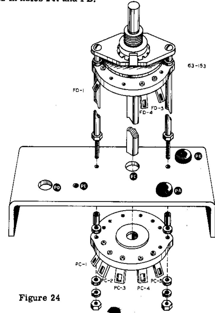
ing holes at FN and FJ. Use lockwashers under the nuts. Now place a 3/8" nut on the switch bushing and secure.
