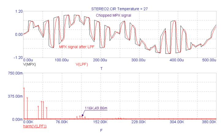
The smoother red line in the top chart is the MPX signal after it has gone through a very simple multistage RC Low Pass Filter. At the bottom, we see the harmonic content of the MPX signal after the LPF. We can see much lower harmonics around 114 KHz while all other higher harmonics have been almost totally suppressed. However the LPF has introduced enormous phase shifts, more about which follows later. A better LC LPF could have been used instead for better results.
