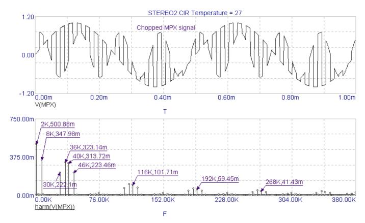
Here we show on the top, the original chopped MPX signal. At the bottom is the harmonic analysis of the same signal. We can see the 2 KHz and 8 KHz signals in the L+R part of the MPX. Further on we see, centered around 38 KHz, the side bands of the L-R signal. The original 8 KHz signal transforms to 38-8 = 30 KHz and 38+8 = 46 KHz signals. Similarly the 2 KHz signal transforms to signals of 36 and 40 KHz. The 38 KHz carrier signal is most obvious in its absence.
