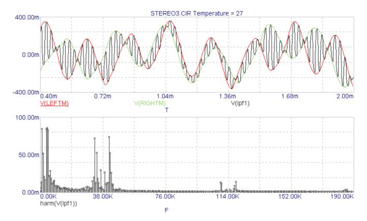
The Black line in the top half is the basic chopped MPX signal passed through a LPF, but no Pilot Tone has been added. In the Harmonic Analysis graph, we can easily make out the L+R region between 0 and 15 KHz, followed by the L-R region between 23 to 53 KHz.
