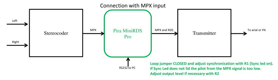
Adjustments of the Synchronization are ideally done with an oscilloscope or else adjust for minimum sound distortion.
