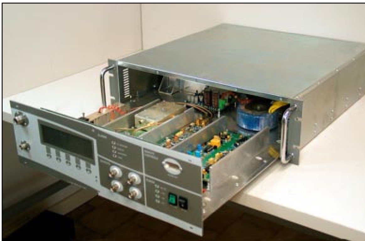
View of the receiver with sliding chassis
