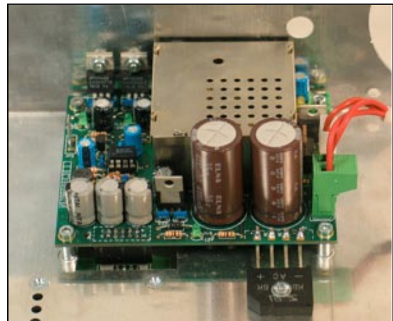
RECEIVER extractable chassis: power supply board in particular
