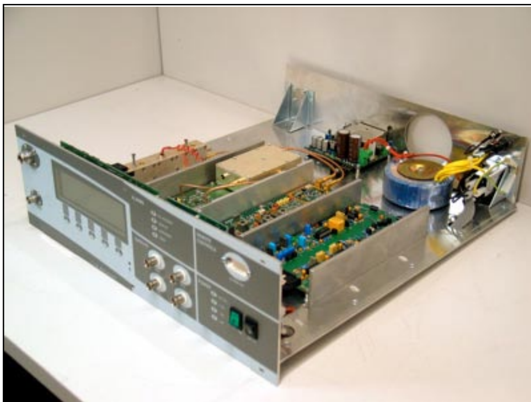
View of the extractable chassis with modules
