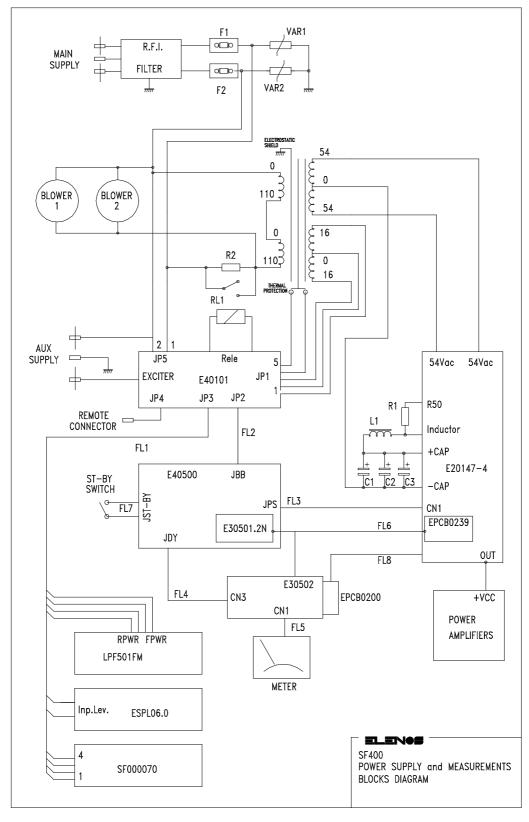
POWER SUPPLY and MEASUREMENT BLOCK DIAGRAM
