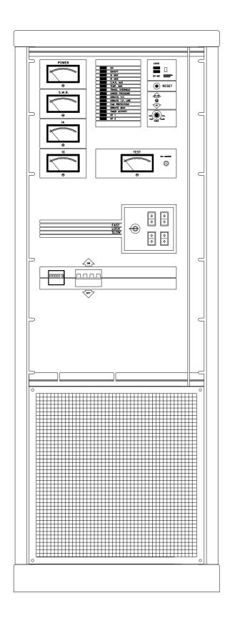
The T10000 is a power triode amplifier conceived for the FM band 88 - 108 MHz, with input and output frequency tuning.
