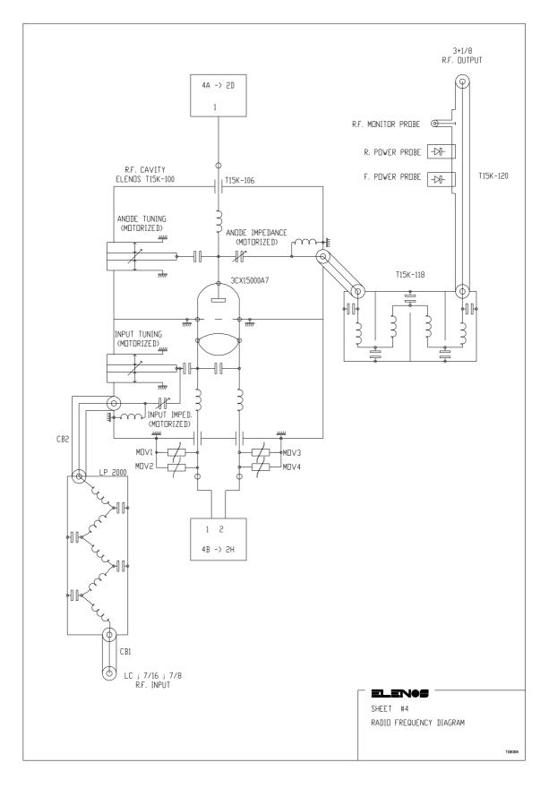
Sheet #4 - R.F. Cavity Amplifier Diagram
