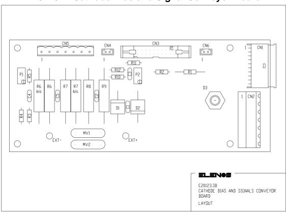
E20123 - Cathode Bias and Signal Conveyor Board
