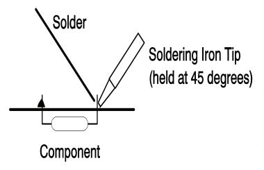
solder directly on the iron from one point. Instead, be sure to use thin solder. Lastly, snip off the excess lead tails less than 1/8 inch or as close to the tip of the cone as possible. **Important.** In R.F. construction, solder components as close to the board as possible, unless otherwise instructed, or the circuit will be prone to instability due to extra lead length adding spurious inductance and capacitance..
