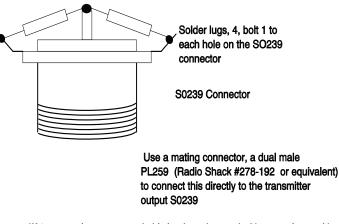
\*If 2 watt resistors are used, this load can be used with transmitters with an ouput power of 5-6 watts maximum.
