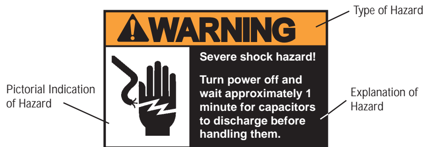
Illustration 1–3 Sample Hazard Alert
