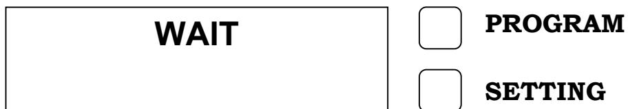
After 3 seconds the green PLL LOCK led will light and the Display will show an increasing bar. After a further 5 seconds the green ENABLE will light and there will be output power.
