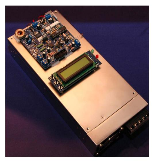
Fig.1: Universal Amplifier Control Board 2.0
