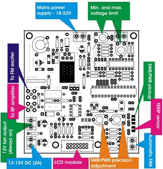
Fig. 4: Amplifier Control Board v20 quick reference
