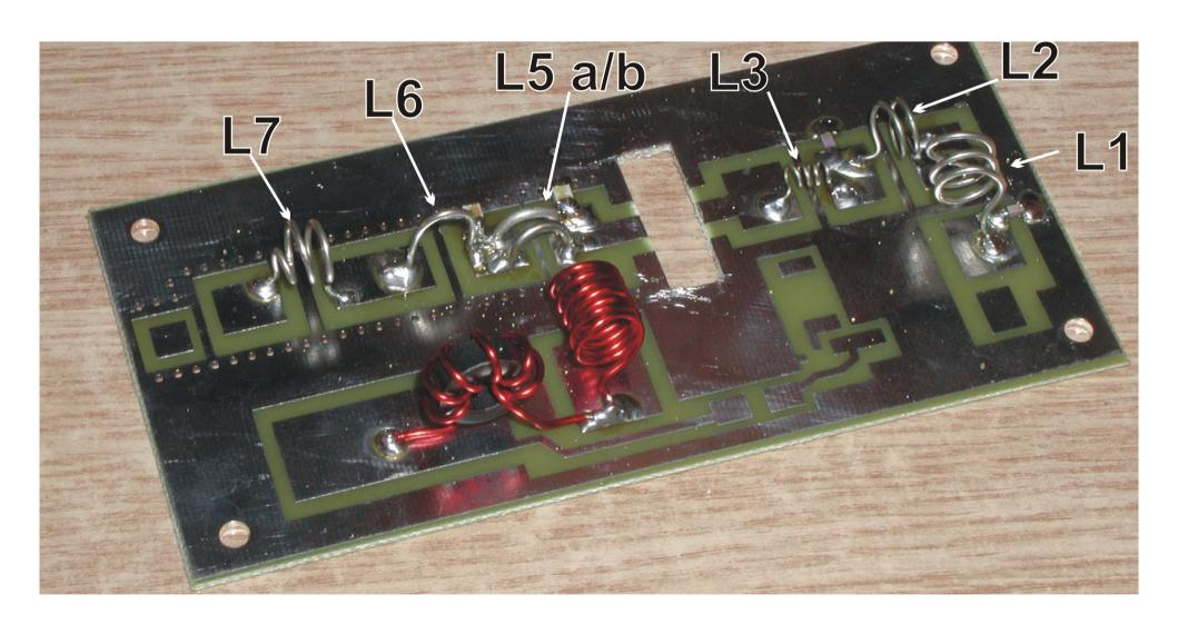
Correct Placement and Soldering of the 40 Watt Amplifier Coils and Inductors
