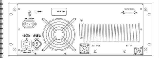
The rear panel allocates the RF power and the I/O ports in addition to the mains power cord and fuse, the earthling screw and an auxiliary mains socket on some models. The power cord is not removable. If it is required a longer cable than that provided in the factory (roughly 2 meters long), a suitable 3x 1.5 mm sq. power cord may easily replace the original one. The fuse has a different rating for 115 or 230Vac operation: be sure to adopt the right type for your mains network
