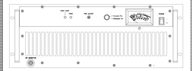
The front control panel carries the power on switch, the control meter, some alarm warning led's and a RF monitor connector. On the bottom side, a gridding on the panel permits the output of the ventilation air.
